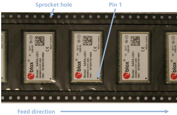
Figure 16: Orientation for SARA-U2 series modules on tape
