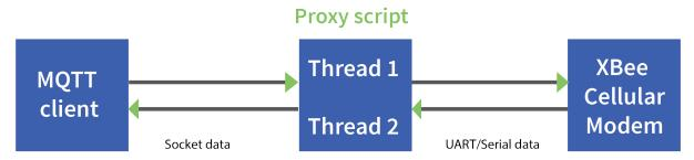
The thread that reads the serial port forwards any data received onward to the client socket, and the thread reading the client socket forwards any data received onward to the serial port. This is represented in the figure above.
