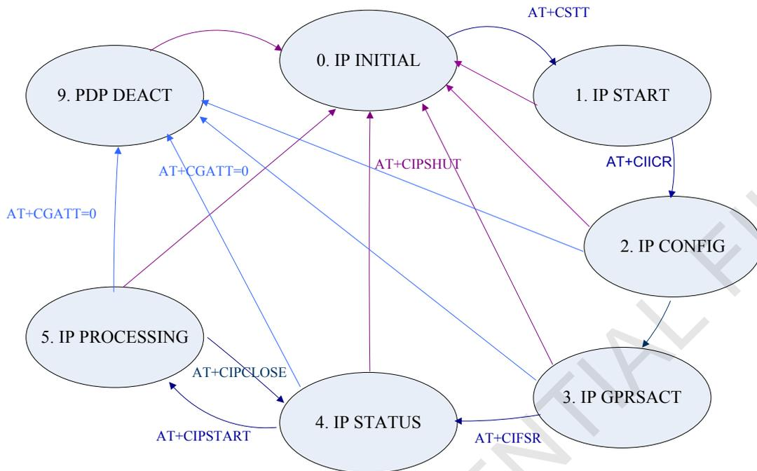
**Figure3: APPTCP States Diagram for multi connection**
