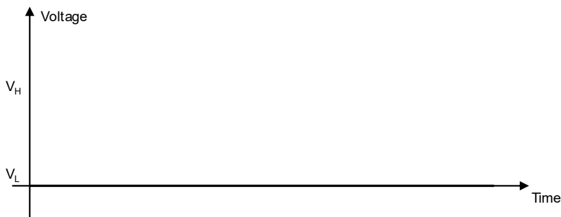
Figure 4: GPIO pin progress for no service
