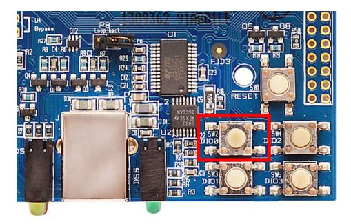
On the board you see **DIOO** written below **SW2**, to the left of the button. This represents the pin that the button is connected to.
