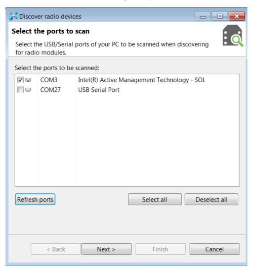
4. Remove the development board from the USB port and view which port name no longer appears in the **Discover radio devices** list of ports. The port name that no longer appears is the correct port for the development board.
