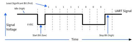
You can configure the UART baud rate, parity, and stop bits settings on the device with the **BD**, **NB**, and **SB** commands respectively. For more information, see Serial interfacing commands.
