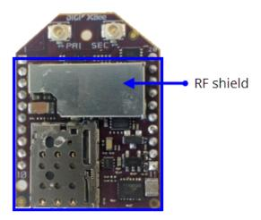
When attaching to the host PCB, tighten the mounting hardware until the gasket is compressed at least 25% and the heat sink is snug against the RF shield. Avoid overtightening. To prevent shorting, check that the surface of the heat sink does not directly contact any of the XBee device components.
